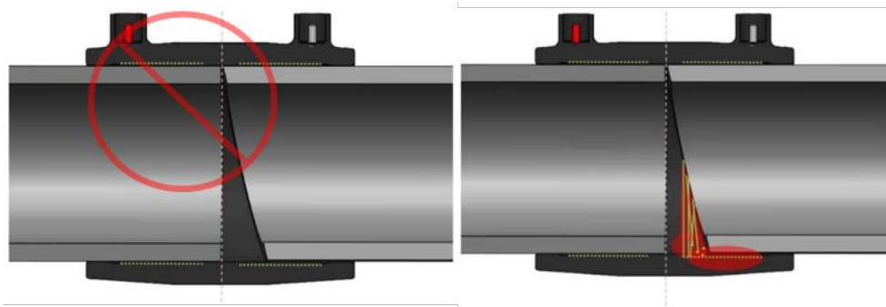
Figure 39: Mis-Cut - Incorrect Assembly
